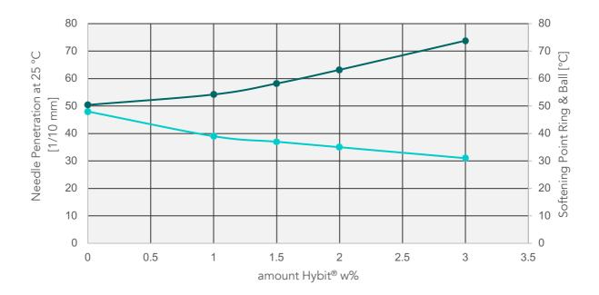
With increasing amount of Hybit<sup>®</sup> the needle penetration drops to lower values and the Softening Point ascends. In fact you get a more durable asphalt which is more resistant to daily stress cause through traffic and different weather conditions. The decreasing of the viscosity leads to a better handling at lower temperatures.
